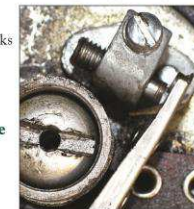
Figure 2. The points block was not aligned with the breaker arm.
